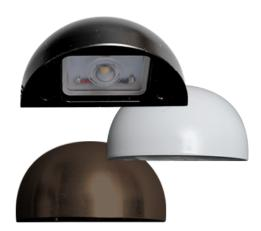
Meridian integrated LED micro-deck lights are crafted from cast aluminum and come powder-coated in black, bronze or white. 1 watt, 12 volts, 3000K warm hue. Easy flush mount. IP65 weatherproof.
